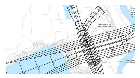
143. OLS are a fundamental requirement in civil aviation to ensure the safety of aircraft operations by defining the airspace that must be free of obstacles. They are legally
