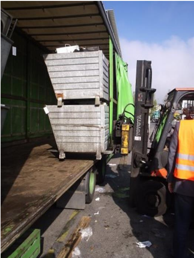
Figure 16: Standardised Bins Being Loaded onto Curtainsider Truck
