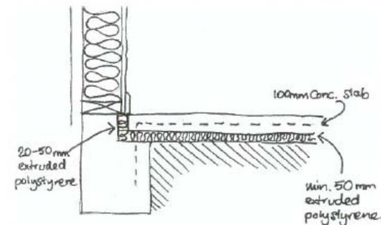
*A method of insulating a slab edge*
