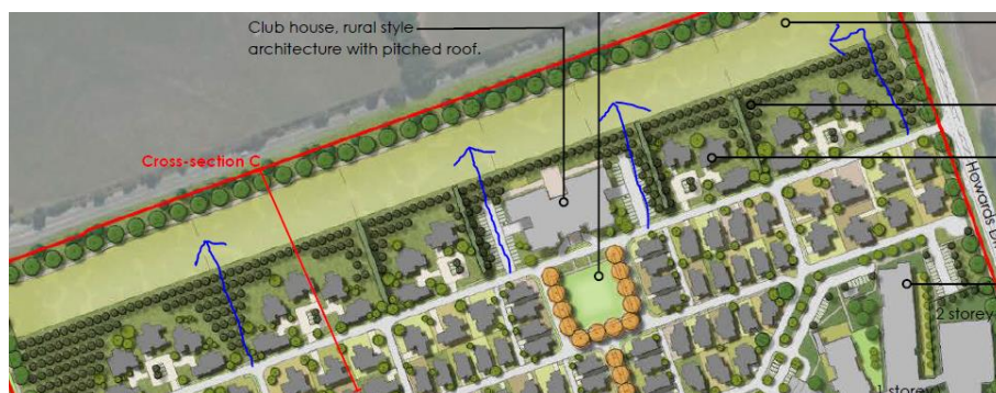
Figure 3: Snip of QCC Master Plan with "blue arrows" indicating how the grid pattern can be modified to provide for future development within the setback area (source: QCC Master Plan from Design Statement for QCC, 14 September 2016).
