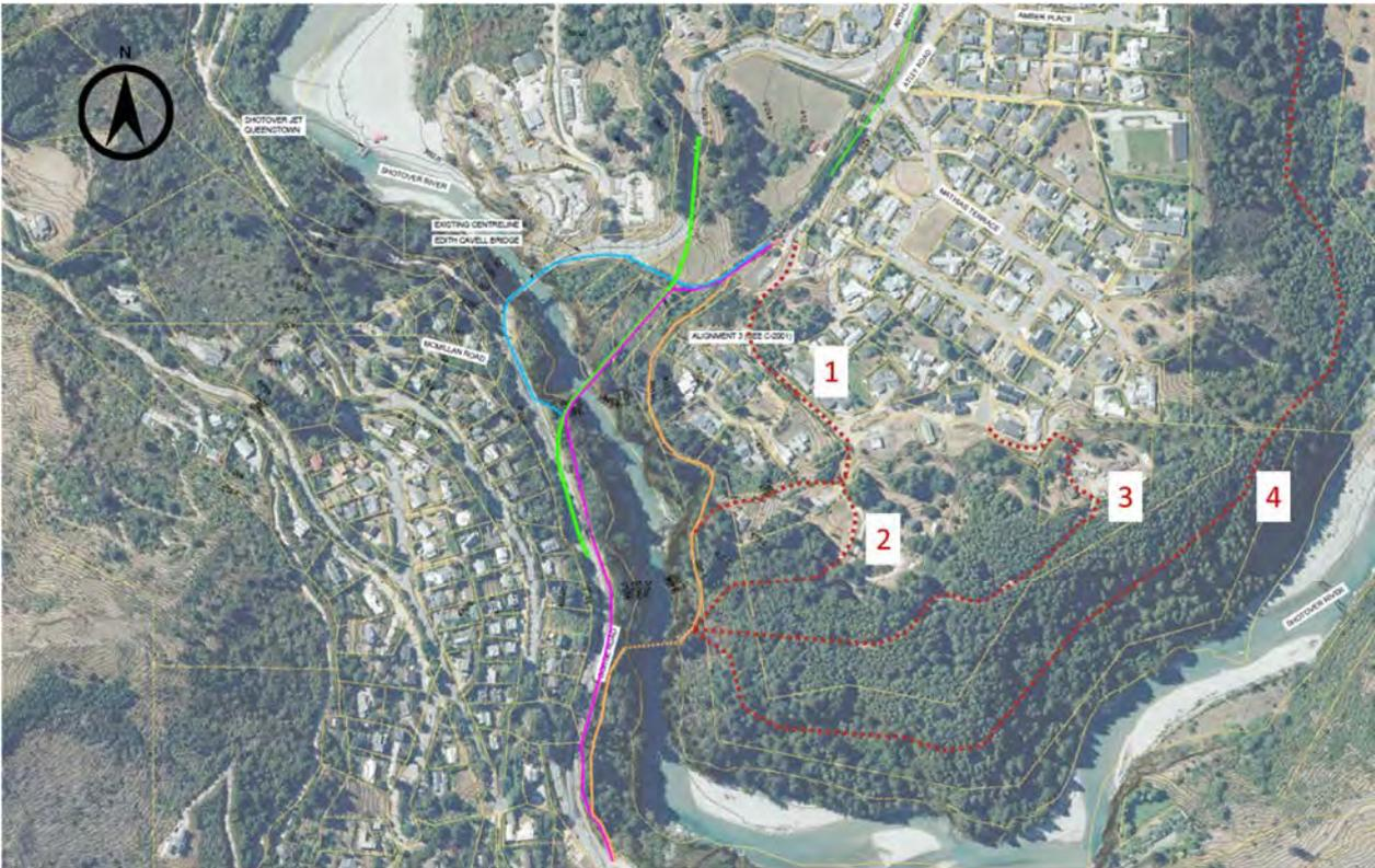
Figure 18 Alternative Active Mode Trail Alignments
