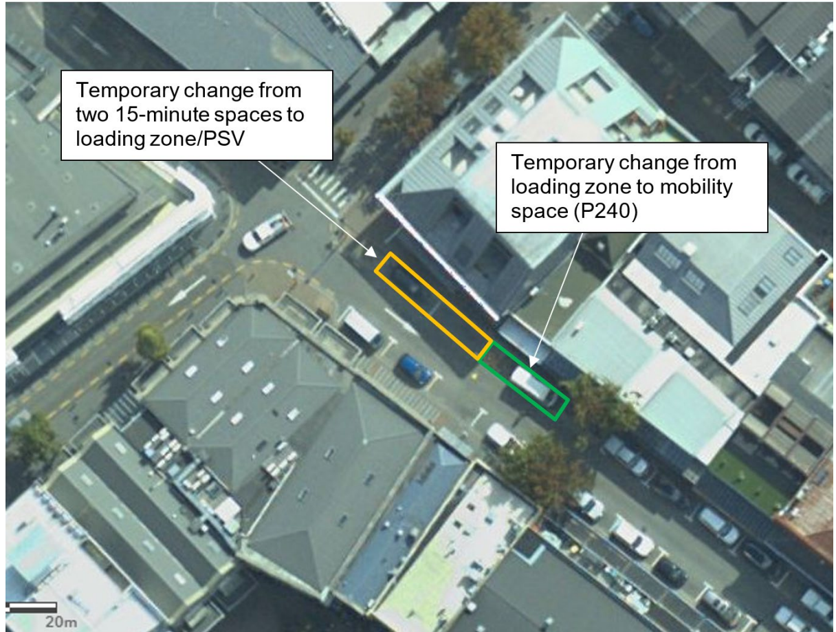
Figure 2. Temporary provisions Rees St
