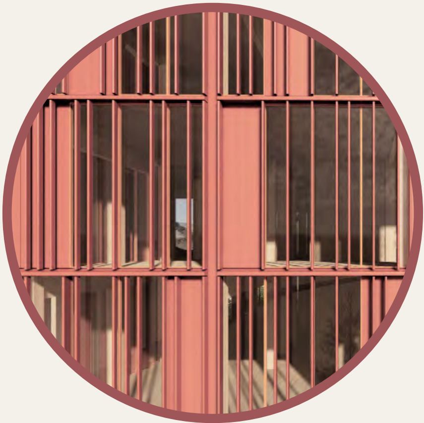
60% glazing with vertical shading to North and South Facades
