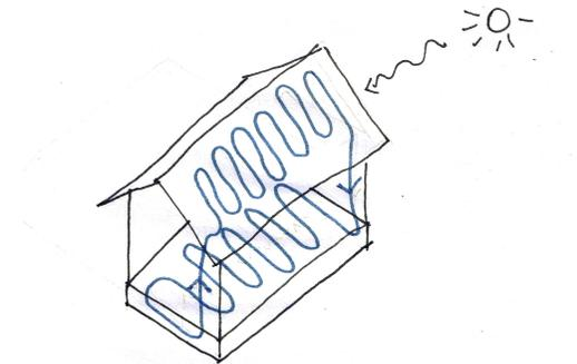
In-slab solar heating
