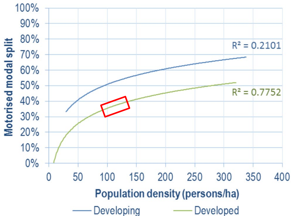
Figure 2 – Public transport motorised modal split for developing (n=24) and developed (n=104) cities from Cooke and Behrens (Note the green line is the relevant part for NZ where GDP/person > US$10,000) Red Box added
