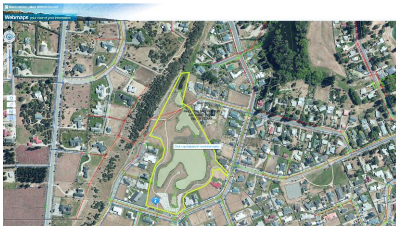
Figure 1 – Subject Site Showing Existing Services (Detention and Treatment Ponds Shown Green). Source – QLDC Website 05.03.15
