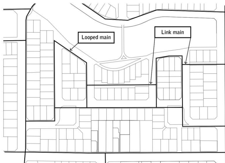
Figure 6.4 – Elimination of termination points
