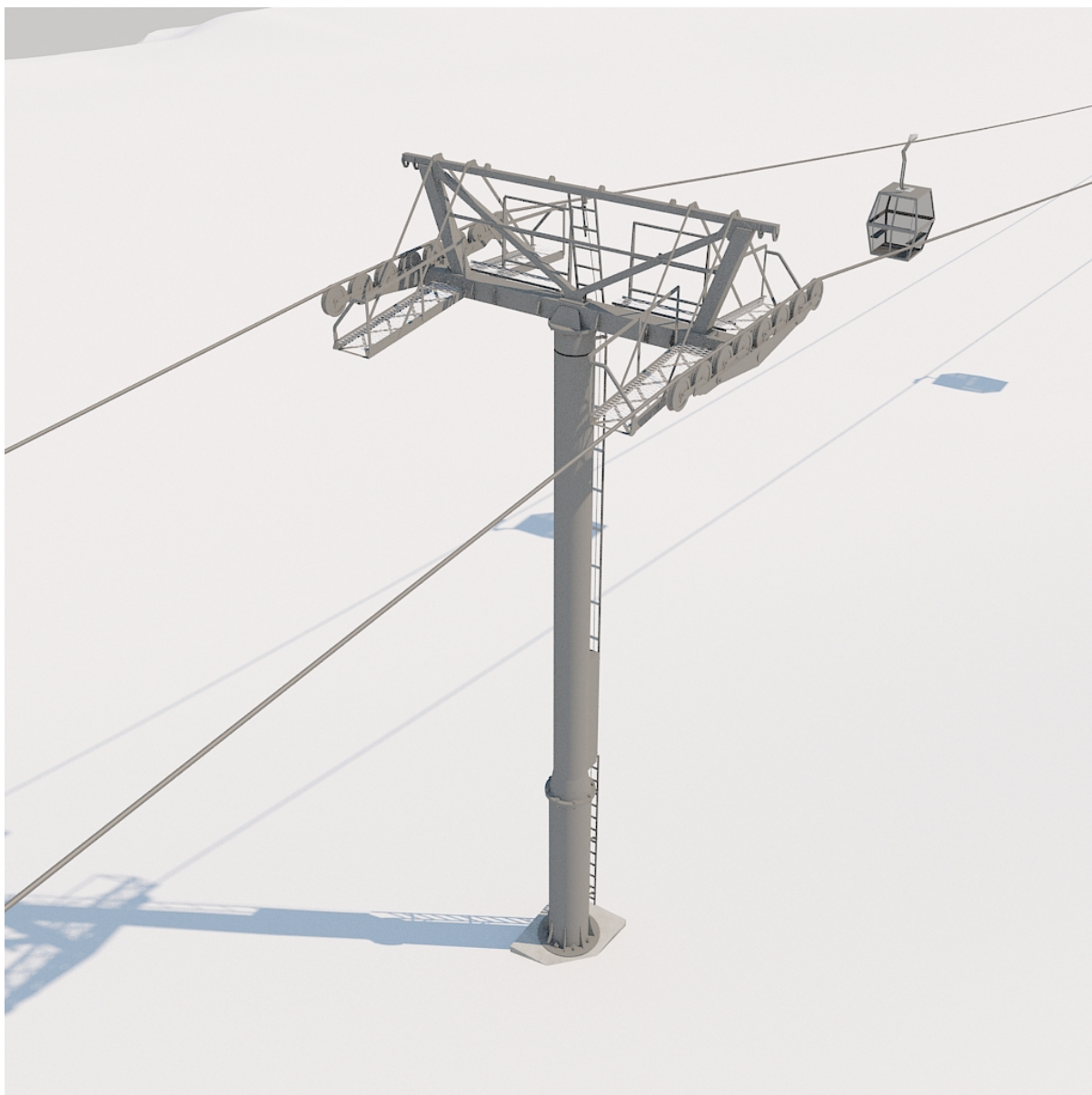
14.1 Figure 1 Gondola Tower.
