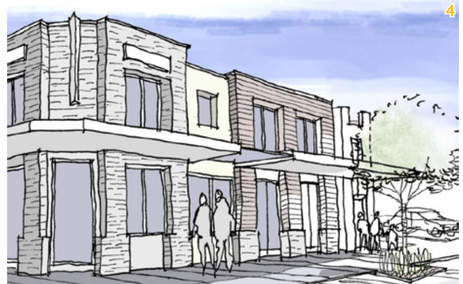
Articulation of verandas corresponds to articulation of building façades
