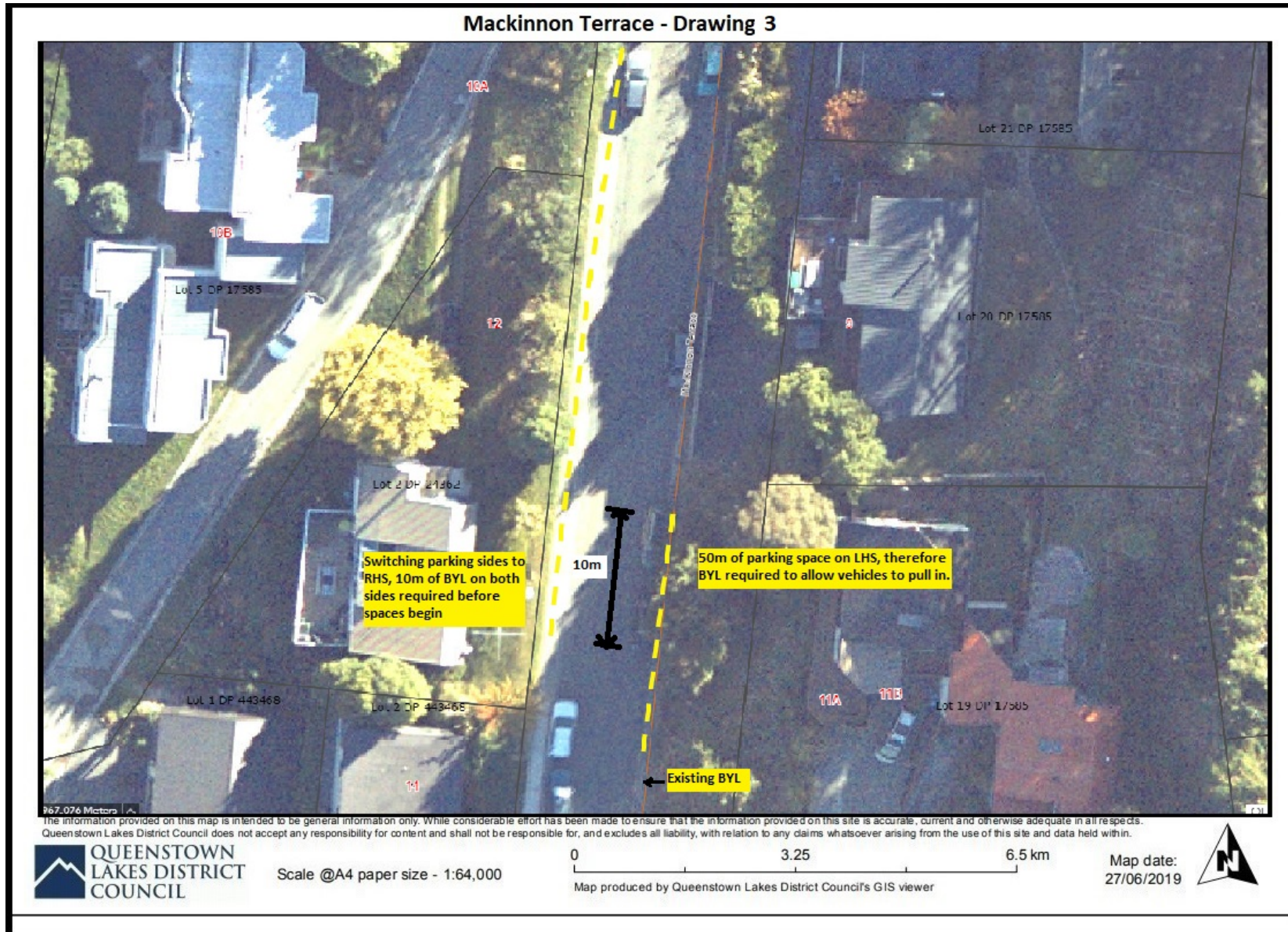
Figure 8: Mackinnon Terrace: No stopping at all times
