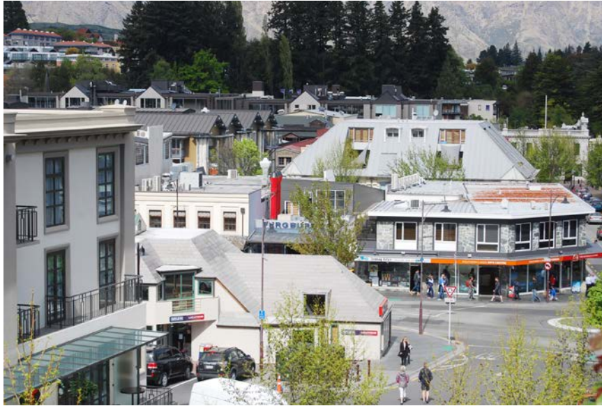
View of town centre from above (Man Street) – Note mixture of roof heights and roof forms from flat to gabled to steeply pitched, exposed and concealed services, colours and eaves treatments.
