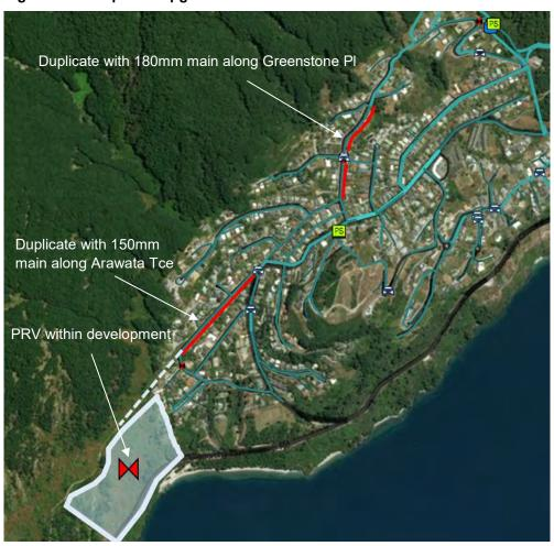
Figure 4-4 - System Performance with Proposed Upgrades - 2058 Peak Day
