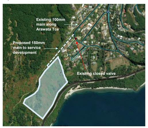
Figure 2-1: Development Connection Configuration
