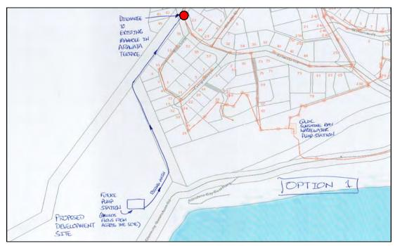
FIGURE 3-2 SUNSHINE BAY OPTION 1 - PROPOSED WASTEWATER NETWORK CONNECTION
