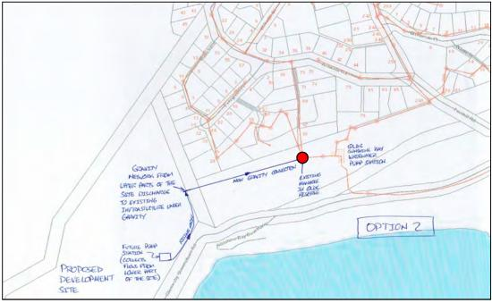
FIGURE 3-3 SUNSHINE BAY OPTION 2 - PROPOSED WASTEWATER NETWORK CONNECTION
