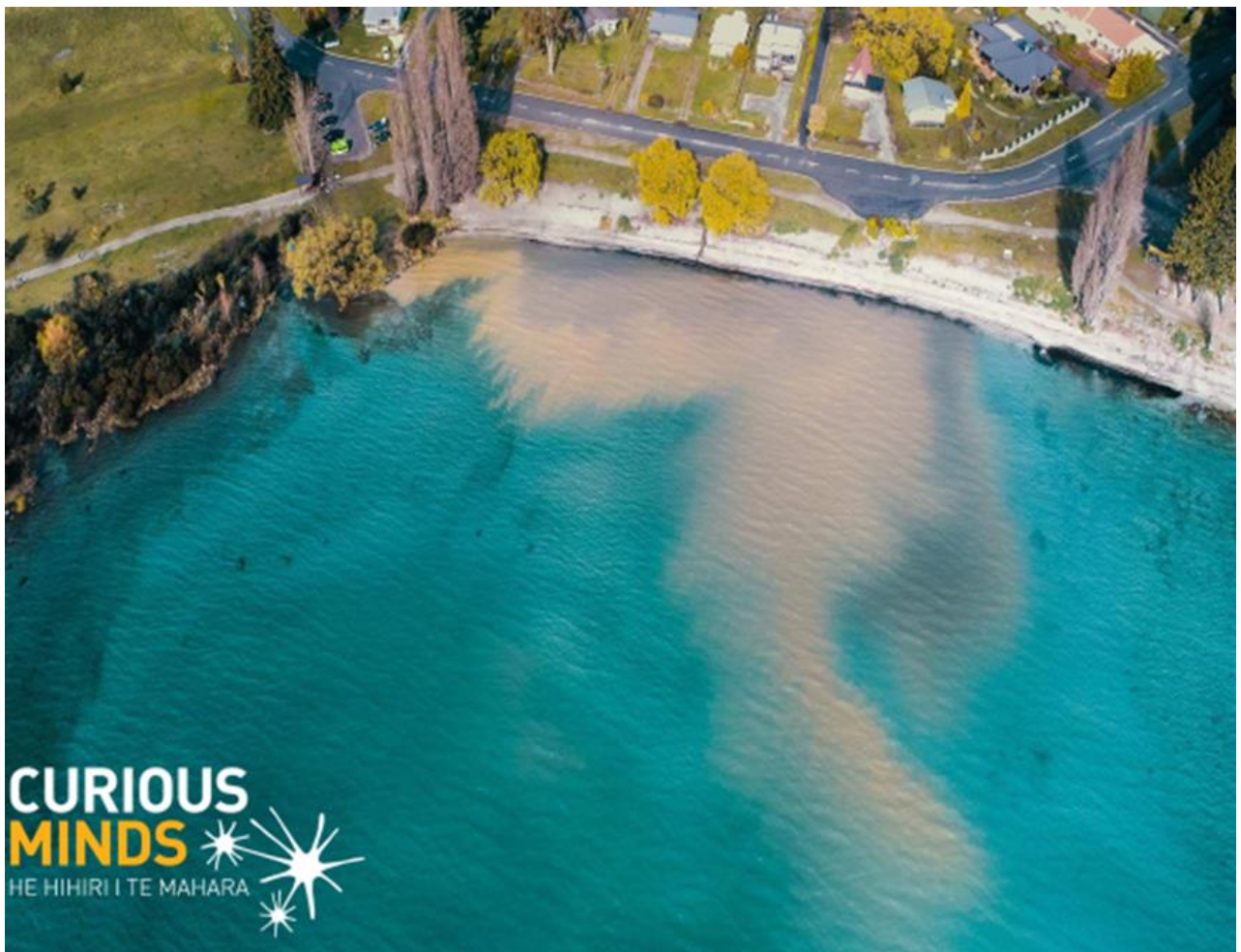
Bremner Bay drain, one of many stormwater sediment flows into the Lake from upstream development.
