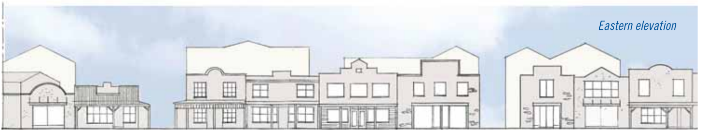
Indicative elevation of what the east side of Cardrona Valley Road might look like with predominantly two storey development along the street frontage built to design guidelines similar to those developed for Arrowtown. Buildings are shoulder to shoulder with occasional gaps indicating alleyways or access to courtyards. Three storeys are permitted set well back from the street front.
